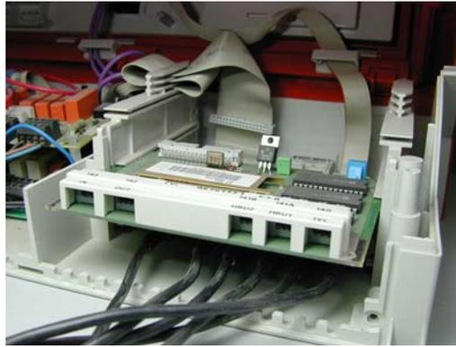
Picture showing communication board sliding into rack above processor board.
