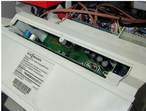
Picture showing the VR20 access into control
