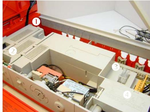
Picture showing 4 clips holding cover over PCB.
