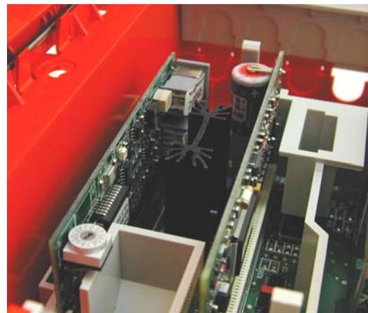
Picture showing installed communication board inside of control. Sockets pointing to rear.
