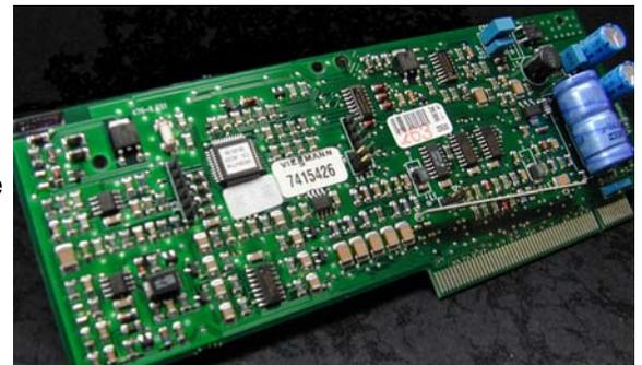
Picture showing VR20 board of the Vitodens boiler.
