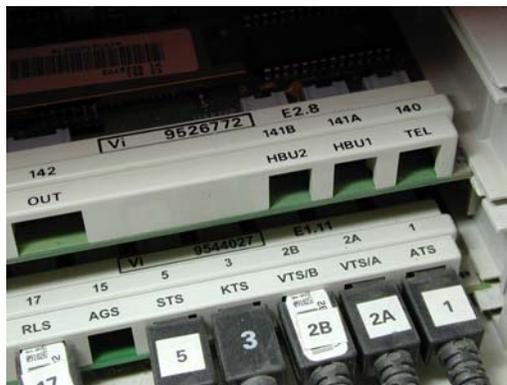
Picture showing communication connection to 141A to Vitocom LON panel.
