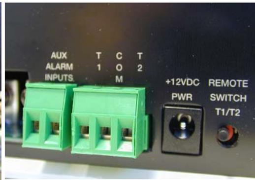
Picture showing Auxiliary alarm inputs, TT connections, power supply and remote switch.
