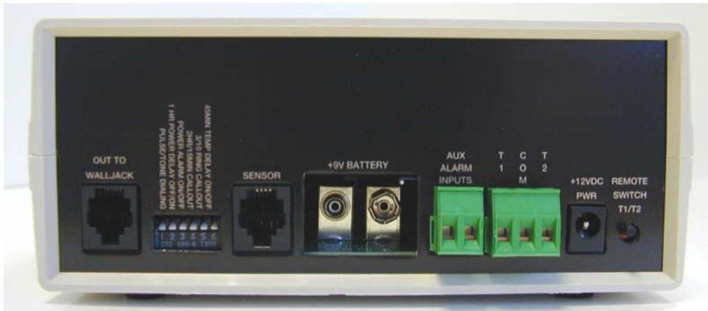
Pictures showing rear of phone dialer plugs and wiring terminals. Note location for 9V battery
