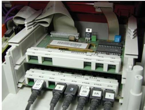
Picture showing communication board pushed in all the way. Ribbon cable plugged in at front.
