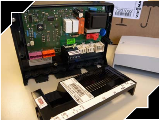
Inside controller with cover removed showing PCB.
